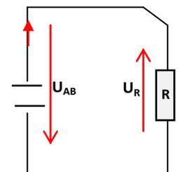
$$i = \frac{dq}{dt} \text{ or } q = Cu_{AB} \Rightarrow i = C \cdot \frac{du_{AB}}{dt} \Rightarrow RC \cdot \frac{du_{AB}}{dt} + u_{AB} = 0$$
